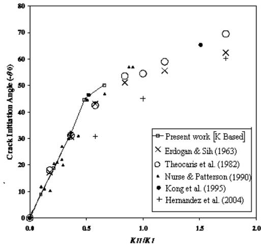
Fig. 1.6: Comparison between crack initiation angle crack initiation of this study and available Ewing *et al.* (1976)
