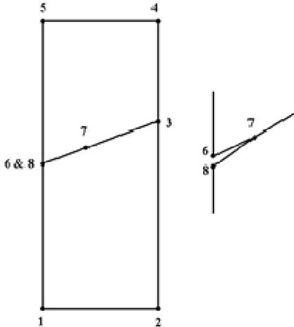
Fig. 1.2: Position of keypoints and lines at crack
