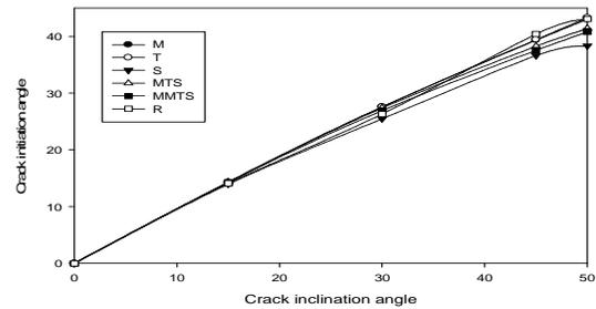
Fig. 1.5: crack initiation criteria at different  $\beta$
