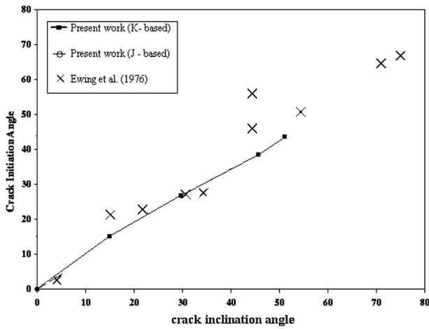
**Fig. 1.7: Comparison between angle of this study and results in the literature**
