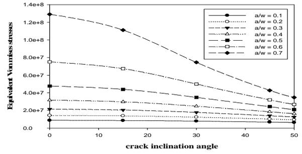
**Fig. 1.8: Von Mises stress at the crack tip**
