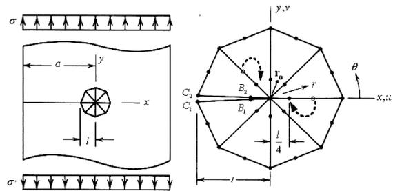
Fig. 1.4: Quarter node element at crack tip
