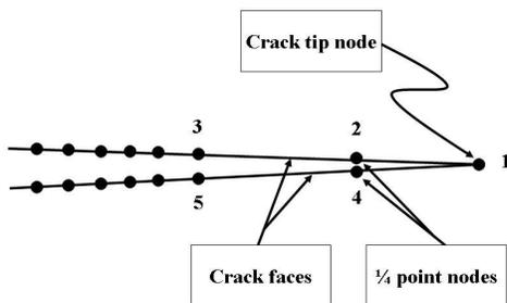
Fig. 1.3: Crack path definition of opening crack
