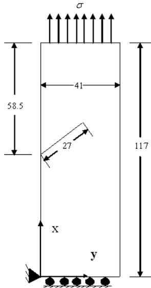
Fig. 1.1: Inclined cracked panel with boundary condition
